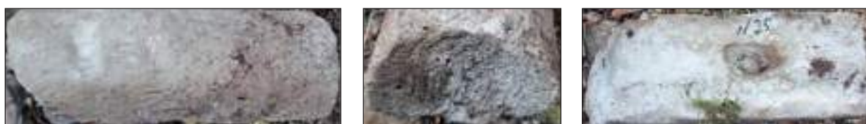
F. N25. The roller of the flagging stone. Flawed. Small hall church (building VI).
